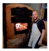
consisting of a double baking chamber furnace with capacity for 70 breads, built on a central metal structure covered with adobe.
